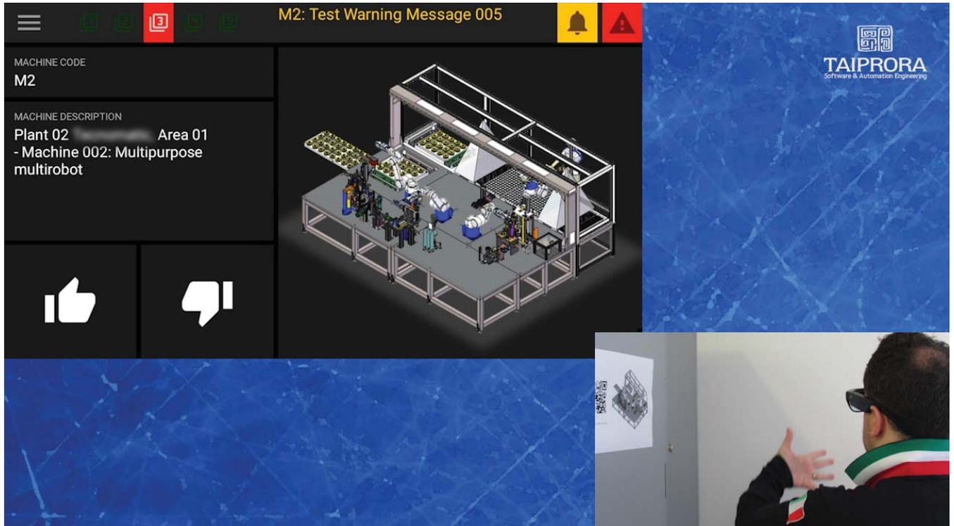
*The operator reading the barcode of the machine through the smartglass camera can access the available features such as maintenance, the status of the sensors, the maintenance operations to be carried out. Moreover, the smartglass alerts in real time on the presence of warnings or alarms inside the system.*
